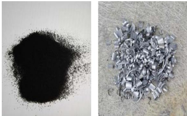
Fig 2. A. Recycled rubber particles. B. Aluminium chips before grinding Material used in preparing the composite mixture
